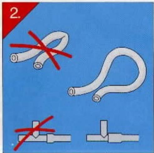
cylinders when they have not been used for some time. To overcome this resistance, work the cylinders a few times by hand before playing with your model until they move smoothly (1). Check that the air tubes have smooth curves and no sharp kinks, which will obstruct the airflow (2).
